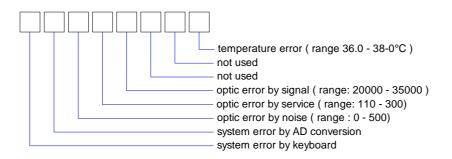
**Example**: The Error Level "00000001" indicates that the temperature is out of range.
