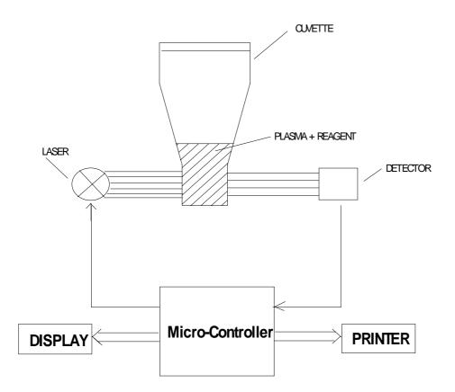
Figure 4 - The detection principle
