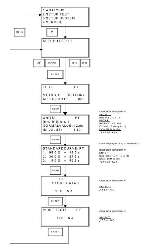
Figure 10 - Flow Diagram for the "Setup Test" Submenu
