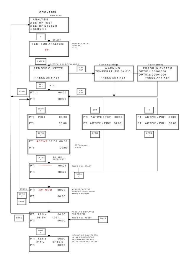
Figure 11 - Flow Diagram of "ANALYSIS" Submenu
