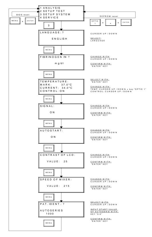
Figure 9 - Flow diagram for the "Setup" System" Submenu
