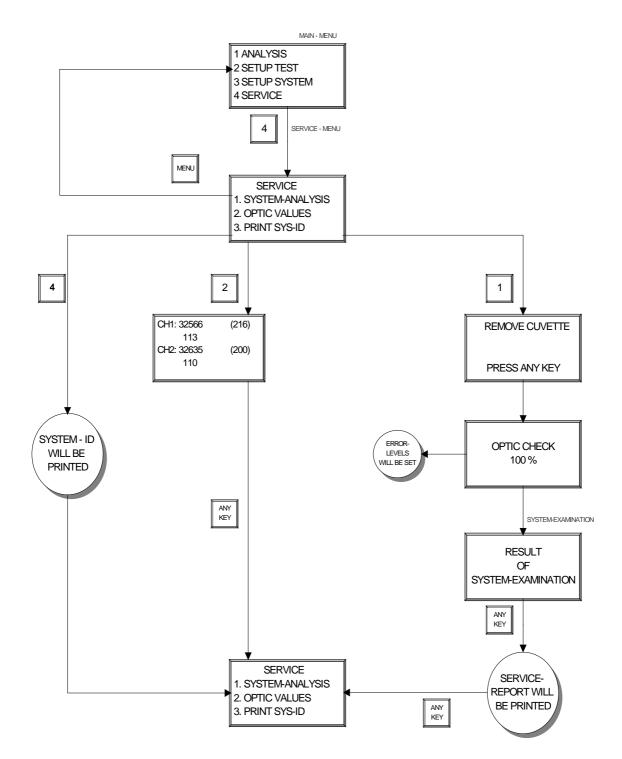
Figure 12 - Flow Diagram of "SERVICE" Submenu
